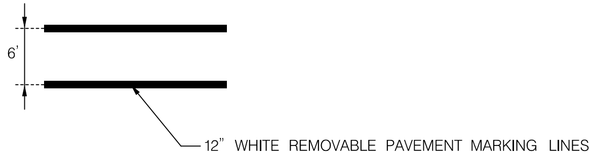
MDOT SHA TEMPORARY CROSSWALK DETAIL (NTS)
