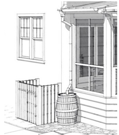
91. Rain barrels help retain stormwater for re-use.
